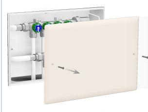
UNSCREW THE FIXING SCREWS OF THE COVER (STANDARD VERSION) INSTALLED ON THE TUTTO PLASTIC BOX AND REMOVE IT
