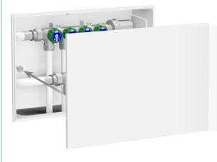
INSTALL THE DESIGNER COVER, MATCHING THE METAL INSERTS ON THE INSIDE, WITH THE MAGNETIC DISCS SCREWED TO THE BOX
